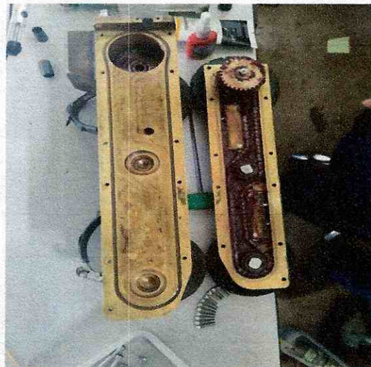
Figura NO.14 o-ring instalado
