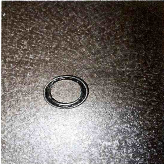
Figura NO.9 seal Deteriorado
